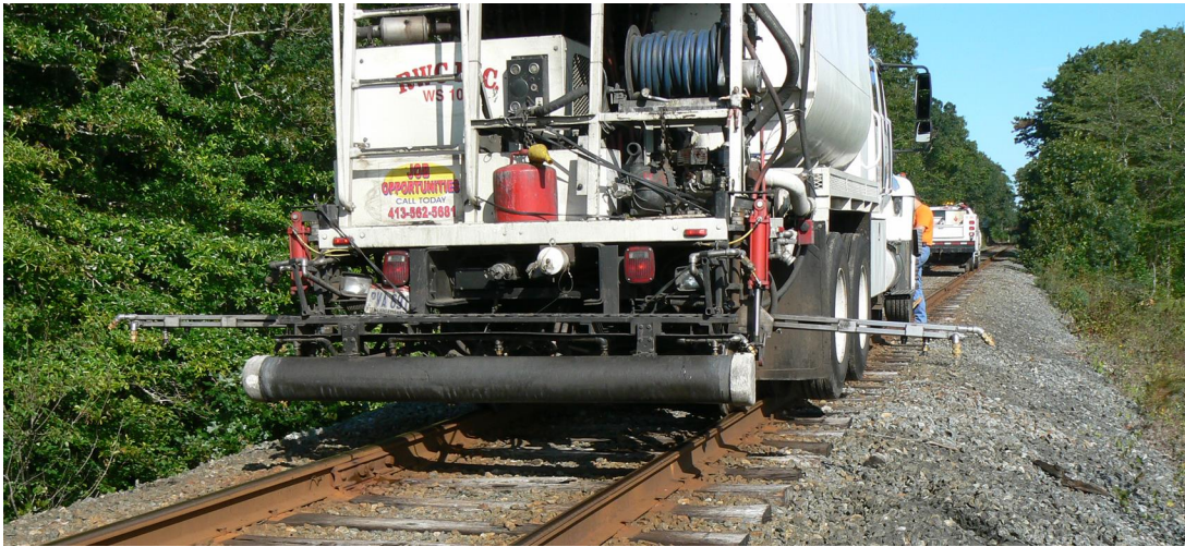
FIGURE 3 REAR MOUNTED BOOM DIAGRAM
